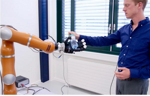
Fig. 9. We evaluated our controller on a KUKA LWR robot equipped with an Allegro hand and the ATI Gamma force/torque sensor, with an Optitrack marker on the human’s wrist. Our approach works with any graspable object with a known mass.
