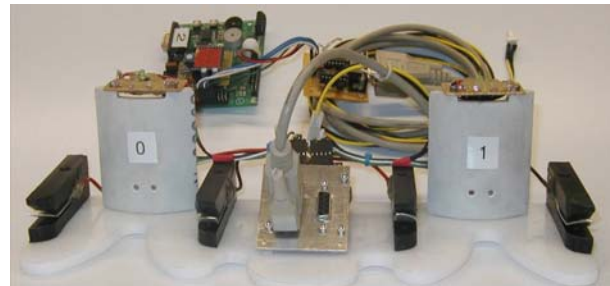
Figure 5: Charging station with two docking bays
