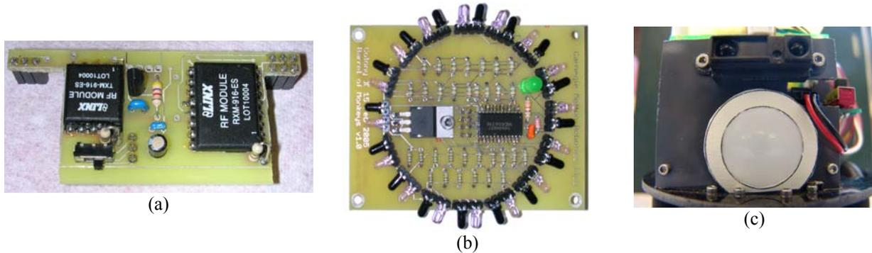
Figure 3.2 (a)The wireless board circuitry; (b)BOM circuit board; (c)Eltec IR-EYE and Sharp GP2D12 IR sensors
