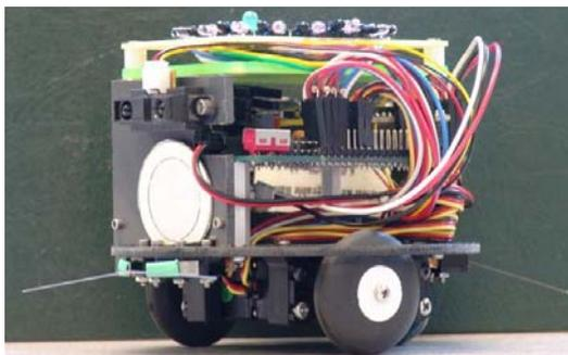
Figure 3.1 One of the colony robots
